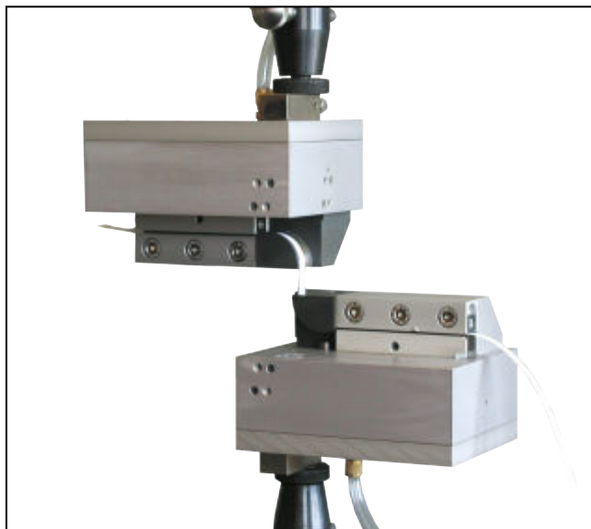
Capstan grips type 8190 Fmax 1 kN, pneumatic
